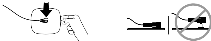
Figure 5-4 Connecting FAST-PATCH Electrodes to Defibrillation Cable
